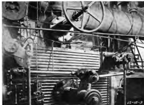
Fig. 3. Guards for Shear-Points in Hooks of Corliss Valve Gear. Fig. 4. Hooks of Corliss Valve Gear with Guards removed.†
